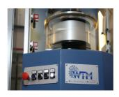
Vertical taping line for mica tape with 1 column with pay-off and take-up for DIN 800 mm. The line is equipped with a double motorized taping head suitable for cross wound spools
