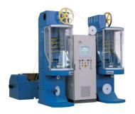
Vertical taping line for mica tape with 2 columns. each equipped with a mechanical taping head suitable for 400 mm pads,
